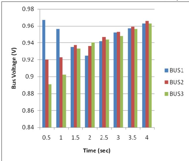
Figure 3: Bus voltages without STATCOM
