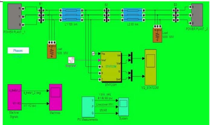
Figure 2: Simulink model with STATCOM
