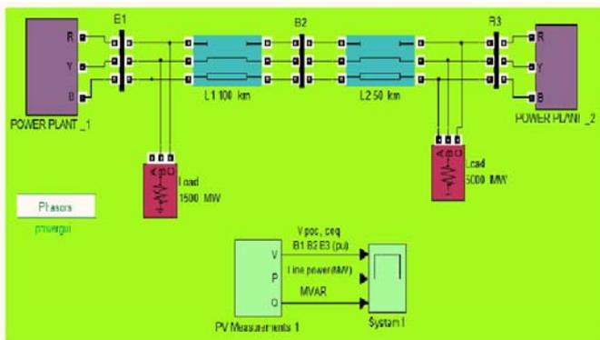
Figure 1. Simulink model without STATCOM
