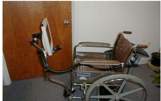
FIGURE 9 : THE PORTABLE EYE GAZE SYSTEM MOUNTED ON A WEIGHS WHEELCHAIR
