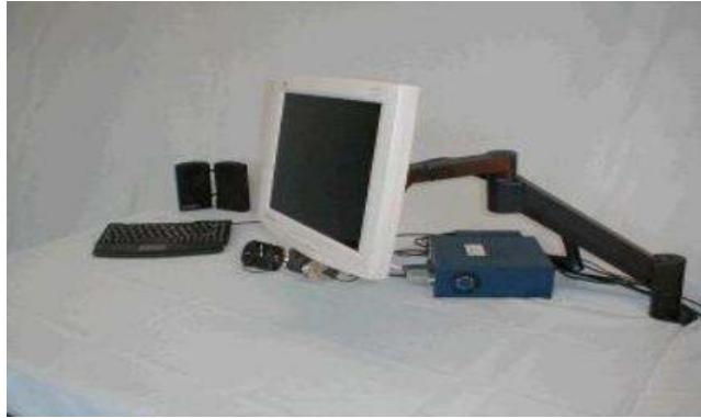
FIGURE 1 : DIRECT-SELECTVISION-CONTROLLED COMMUNICATION AND CONTROL SYSTEM
