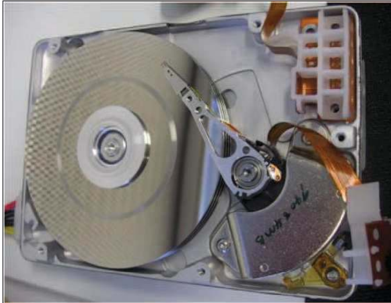
Fig 3.2: The dull ring near the middle diameter of this spinning disk is the result of a head crash.
