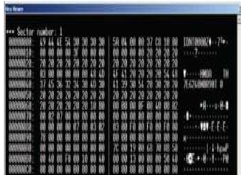
Fig:3.1 The beginning of the identification sector (IDNT) of the system area for a 2.5 Hitachi drive
