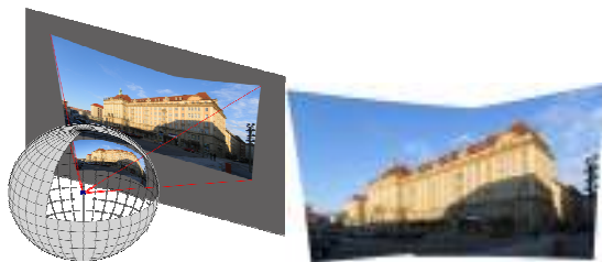
Fig. 8 Projection of sphere image to screen
