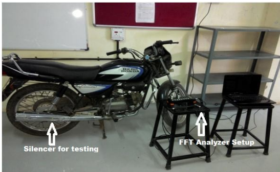
Fig-1-Experimental setup to determine natural frequency
