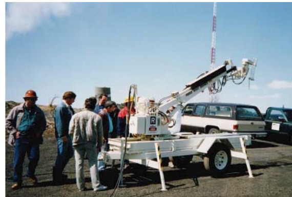
Fig 6: Compact trailer-mounted robot
