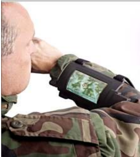
Figure 1. Demonstration of a soldier wearing the wrist unit with a navigation display on.
