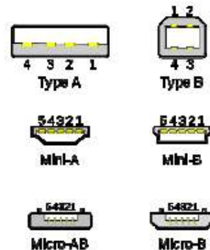
Fig 5.1: Pin outs of Standard ,Mini, and Micro USB connectors
