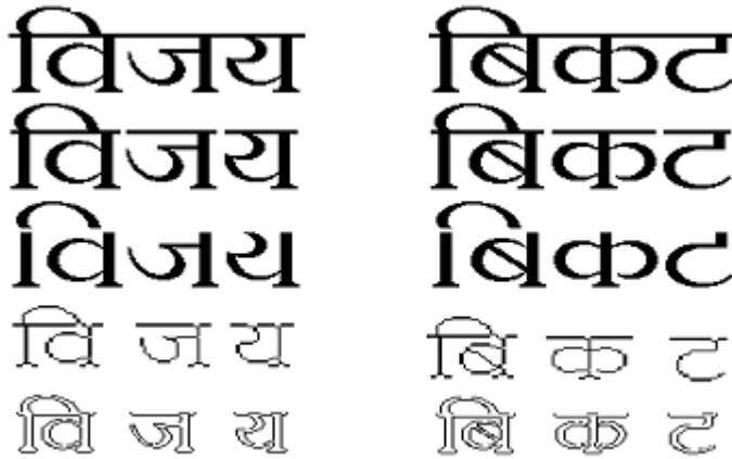
Fig. 3 Preprocessed Images (a) Original (b) segmented (c) Shirorekha removed (d) Thinned (e) image edging
