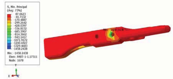
Fig 11 .Results of Maximum principal stress
